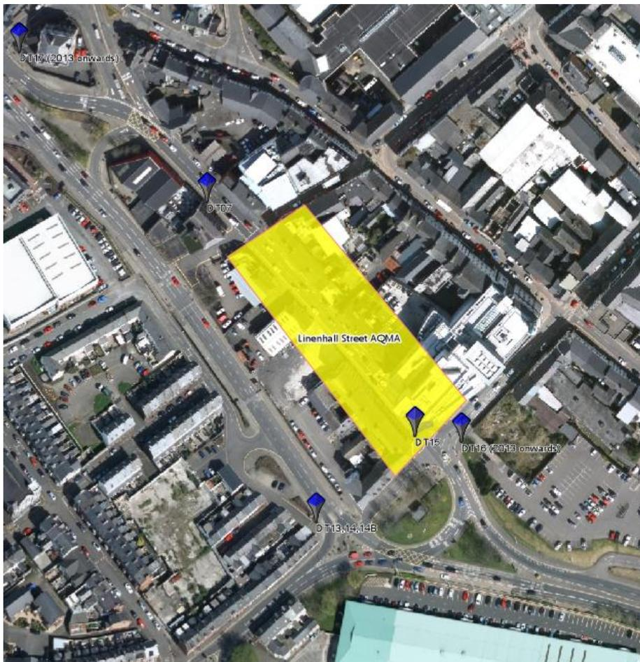
Figure 2-1 Linenhall Street AQMA showing location of Diffusion Tubes
